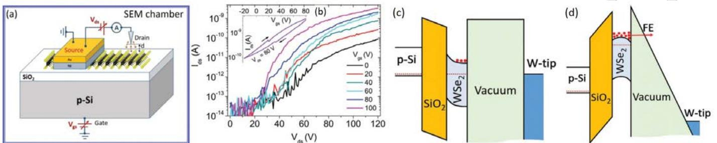
Fig. 1: (a) Layout of a back-gate FE transistor with a WSe<sub>2</sub> monolayer channel over a SiO<sub>2</sub>/Si substrate. The W-tip labelled as the drain, which collects field emitted electrons and monitors the current, is kept at a distance  $d$  from the sample, while the voltage is ramped up. (b) FE current measured at given back-gate voltages ( $V_{ds}$  steps of 1 V). (c) Band diagram for (c) the unbiased device and for (d) the device under  $V_{ds} > V_{gs} > 0$  V bias conditions.
