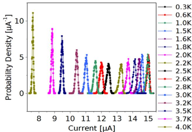
Fig. 1: Measured switching-current distributions for temperatures between 0.3 K (right-most) and 4 K (left-most) that shows the counterintuitive narrowing with increased temperature above 2.5 K.
