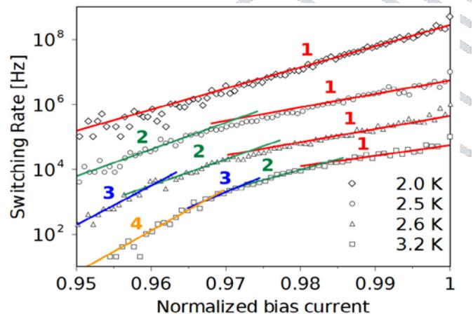
Fig. 2: Switching rates for four different temperatures. The solid lines are fits to the data using the indicated higher order multiple phase slip events included. For clarity we have multiplied both the data and fits by a factor of 10 (2.6 K), 100 (2.5 K) and 5000 (2.0 K) respectively.
