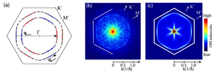
Fig. 1: (a) Fermi surface of Pb- $3\times 3$ /Si(111) including spins polarization (arrows). White arrows, 100% in-plane polarization; blue and red arrows, opposite out-of-plane components. Black arrows are the scattering vectors. (b) Fourier transform map measured by STS at  $T=0.3$  K, corresponding to quasiparticle interference at  $E=E_F$ . (c) Calculated quasiparticle interference map at  $E=E_F$  assuming scalar impurity scattering.
