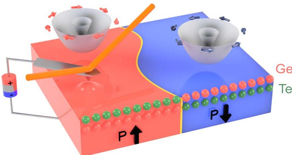
Fig. 1: Switching of GeTe spin texture of Rashba-type for two different orientations of the ferroelectric polarization. On the left (right) region, the polarization is pointing out of (towards) the surface (see vertical black thick arrow denoting  $P$ ) and the spin expectation values at a specific constant energy map, denoted as red (blue) arrows, circulate clockwise (counterclockwise).
