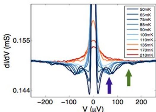
Fig.1: Conductance spectra of a LAO/STO based junction. The arrows indicate the two gap structures
