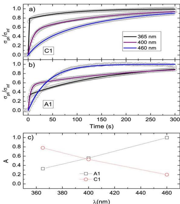
(a) Photoresponse of C1 and (b) photoresponse of A1 at 365 nm (black), 400 nm (red), and 460 nm (green). The data are normalized to the asymptotic value  $\sigma_{inf}$ ; solid lines are fit curves. (c) Dependence of A vs. radiation wavelength  $\lambda$  for both samples.
