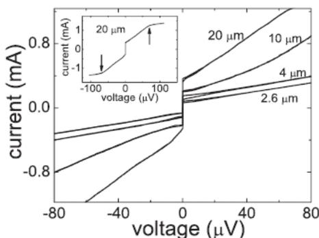
FIG. 1. Current-voltage characteristic of  $45^{\circ}$  [001] tilt bicrystal GBJs with different sizes measured at  $T = 4.2 \text{ K}$ . In the inset, the IV characteristic of a junction  $20 \mu\text{m}$  wide shows peaks due to flux motion.
