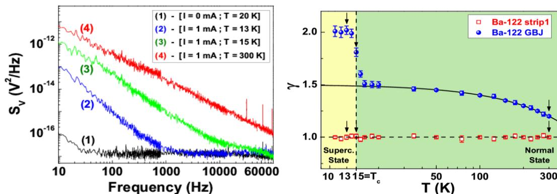
(Left) Frequency dependence of the voltage-spectral density, at three reference temperatures and at a fixed bias current, for the strip containing a grain boundary junction. (Right) Temperature dependence of the noise frequency exponent  $\gamma$ . Red open squares refer to the strip without the grain boundary junction; blue full circles refer to the intrinsic grain boundary junction.
