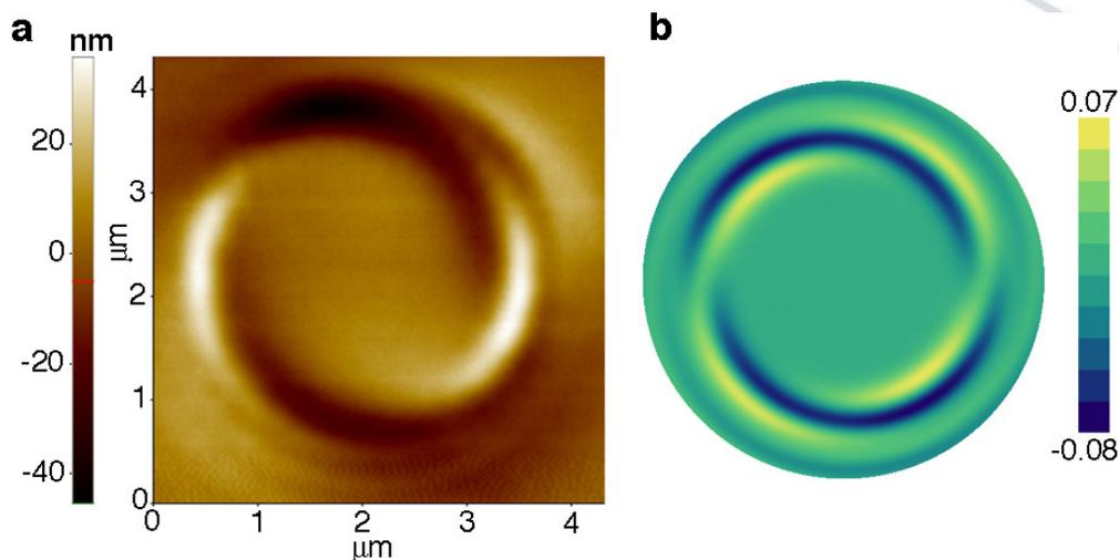
Figure – (a) Relief spiral patterns induced on the polymer by an impinging vortex light beam. (b) Pattern predicted by our model.
