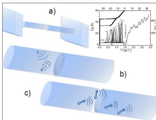
Top right inset: Current-Voltage characteristics. Switching current probability distributions versus bias current for different temperatures down to 300 mK. Resistance versus voltage (voltage scale at the top). a) Scheme of the YBaCuO nanochannel; b) and c) enlargement of grain boundary (GB) region belonging to the nanochannel. Interfering quasiparticles and Cooper pairs transport processes across the GB are sketched in b) and c) respectively.
